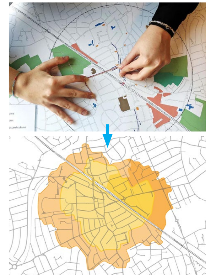
Manually calculating a 'Pedshed' area on a basemap (courtesy of TfL Urban Design)
